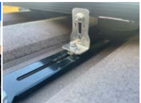
PHOTO 9: Unloaded Bracket - after tests
