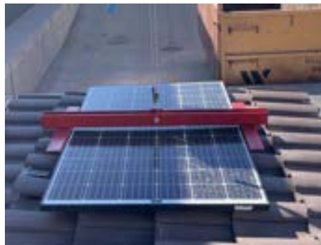
PHOTO 5: Test specimen while under tensile load
